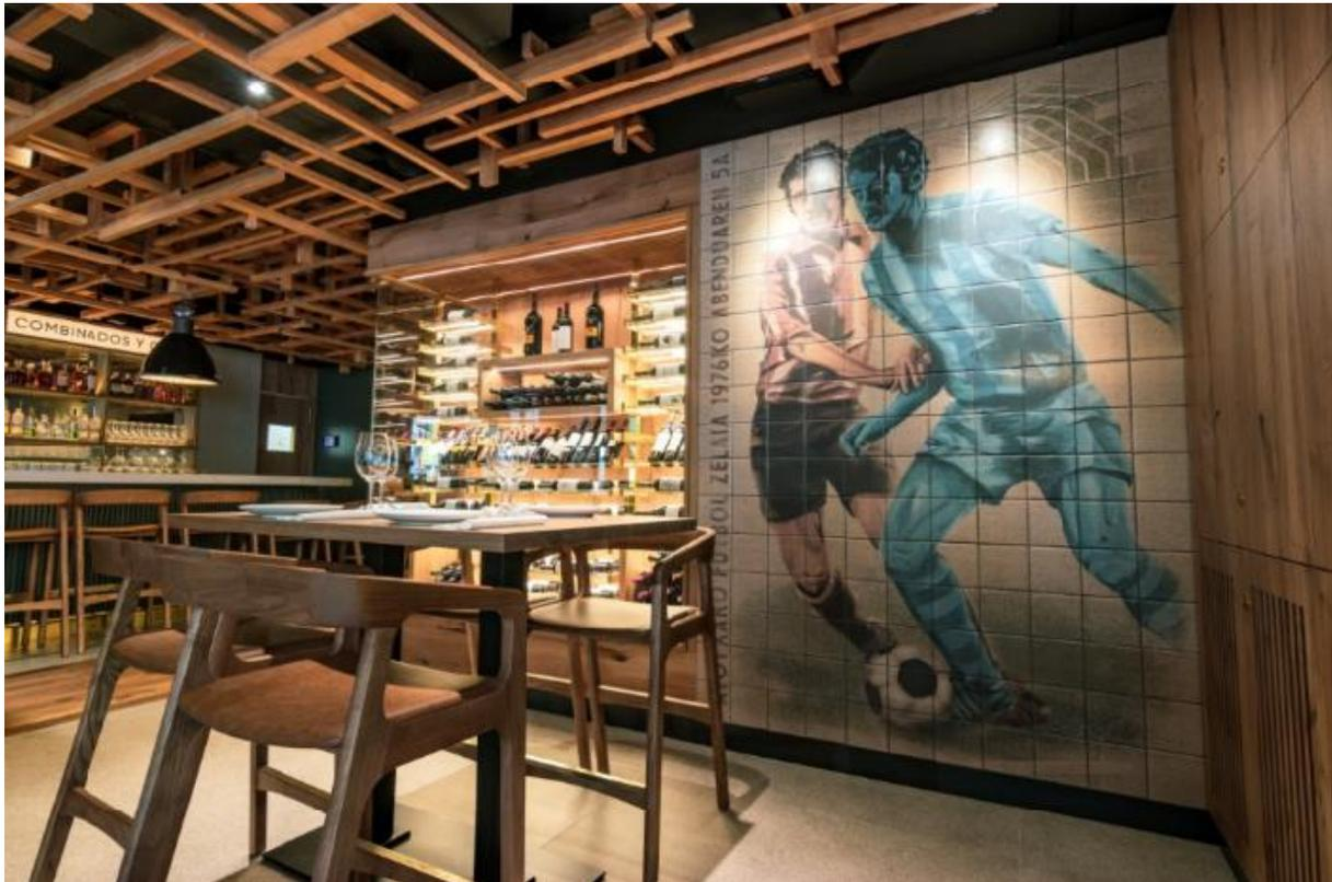
Sublime, the Group Concord company in Mallorca tasked with designing the murals, explains the sublimation process performed on HI-MACS® as a complicated technique, by which **digital prints were transferred in a gaseous state to the solid surface**, by applying controlled pressure and heat in special kilns.
