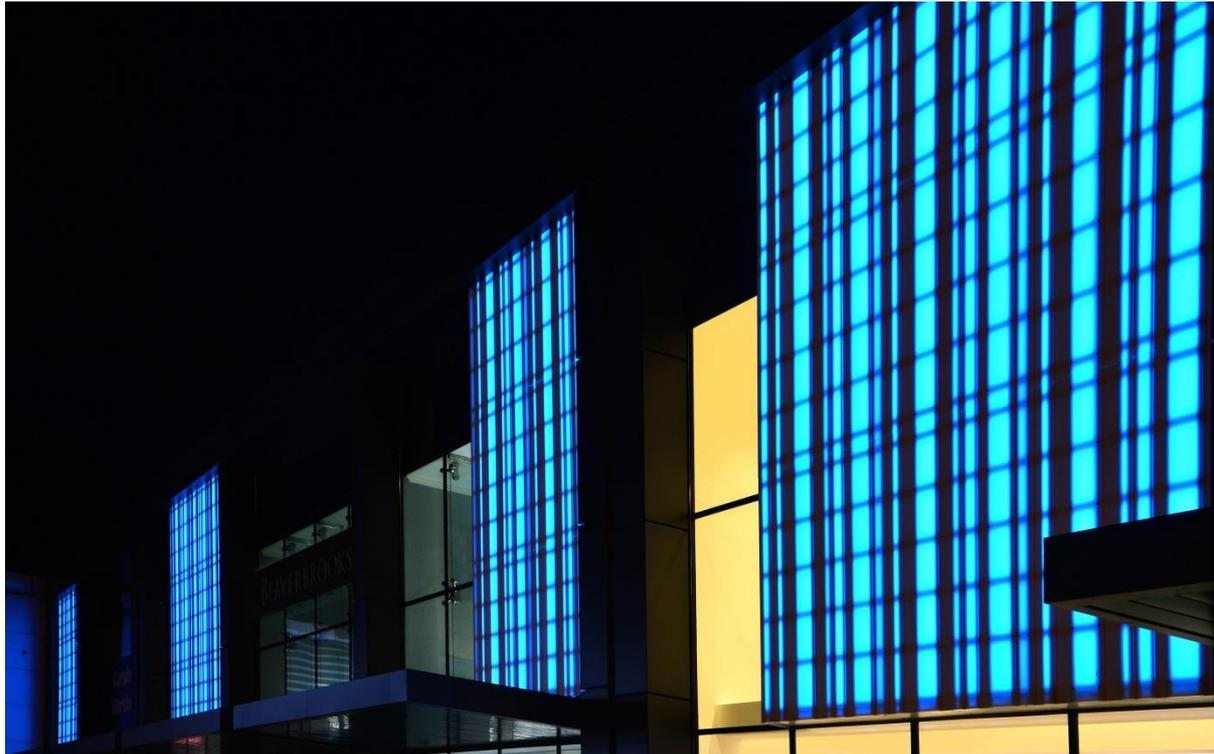
Offering almost infinite design possibilities, **HI-MACS®** is the perfect material for exterior **cladding** and boasts a long list of features and benefits, including three-dimensional thermoplastic forming capabilities and an extensive range of colours. It was particularly selected for this project due to its excellent resistance to weathering and dramatic translucency.
